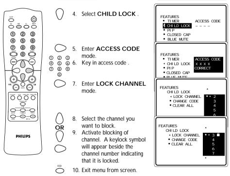
**Note** : You cannot have access to the locked channels via the TV set's controls. You can only have access to the locked channels via the remote control. When AV1 source is locked, CV1 source is automatically locked. Likewise, if CV1 source is locked, AV1 source is also automatically locked, as they share the same audio input.
